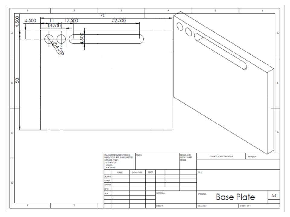
(Length=70 Width=50 Thickness=5) (Material=Aluminium FeedRate=10 ToolDia=4.5)
